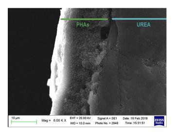
PICTURE: section microscope picture PHAs outside and Urea inside.
